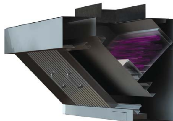
Drawing of UV tubes within the canopy extract plenum
