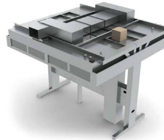
During the design process it became apparent that the existing roof structure would not support the weight of large ventilation canopies, this problem was solved by the use of structural ground support frames, designed and installed by Britannia. All the canopies stand on their own legs, removing the need to reinforce the fragile roof structure.
